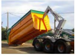
**13h30** Hooking and transport of a grain container to prepare seeding.
