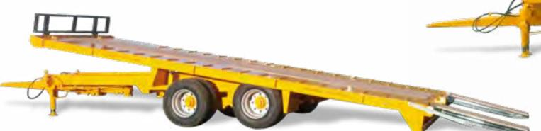
**PEA 240** The tilting bed version of the loader with damping cylinders
